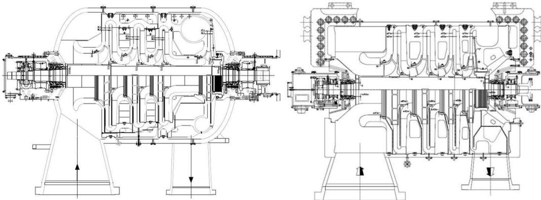
**Figure 7 – Round End vs. Flat End Casing Configuration**
