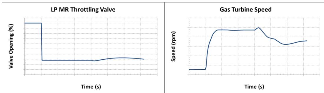
**Figure 9. Companion String: MR Throttling Valve (left) and Gas Turbine Speed (right).**
