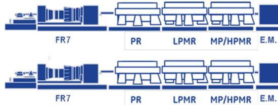
**Figure 3b. New Dominion Compressor Arrangement**
