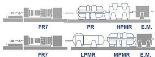
**Figure 3a. Typical Compressor Arrangement**
