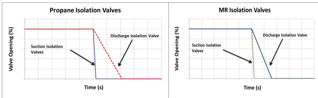
**Figure 8. Tripped String, Isolation Valves: PR (left) and MR (right)**
