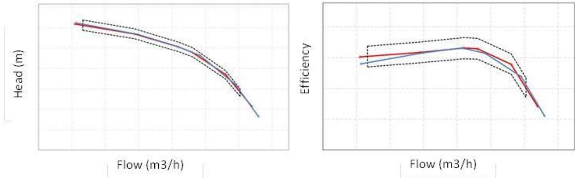
**Figure 6. Head and Efficiency: String A (Red) vs String B (Blue) Including Tolerance Range  $\pm 2\%$  (Dotted Box)**
